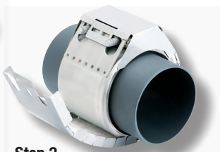
Step 2 Position the flame protection housing over the coupling closure
