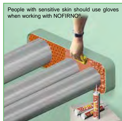
15) A cloth is sprayed with water. Note: do not use soap water! The cloth is used to press down the sealant layer. Pressing down the NOFIRNO® sealant in a stiff way is absolutely vital for the mechanical stability of the sealing system.
