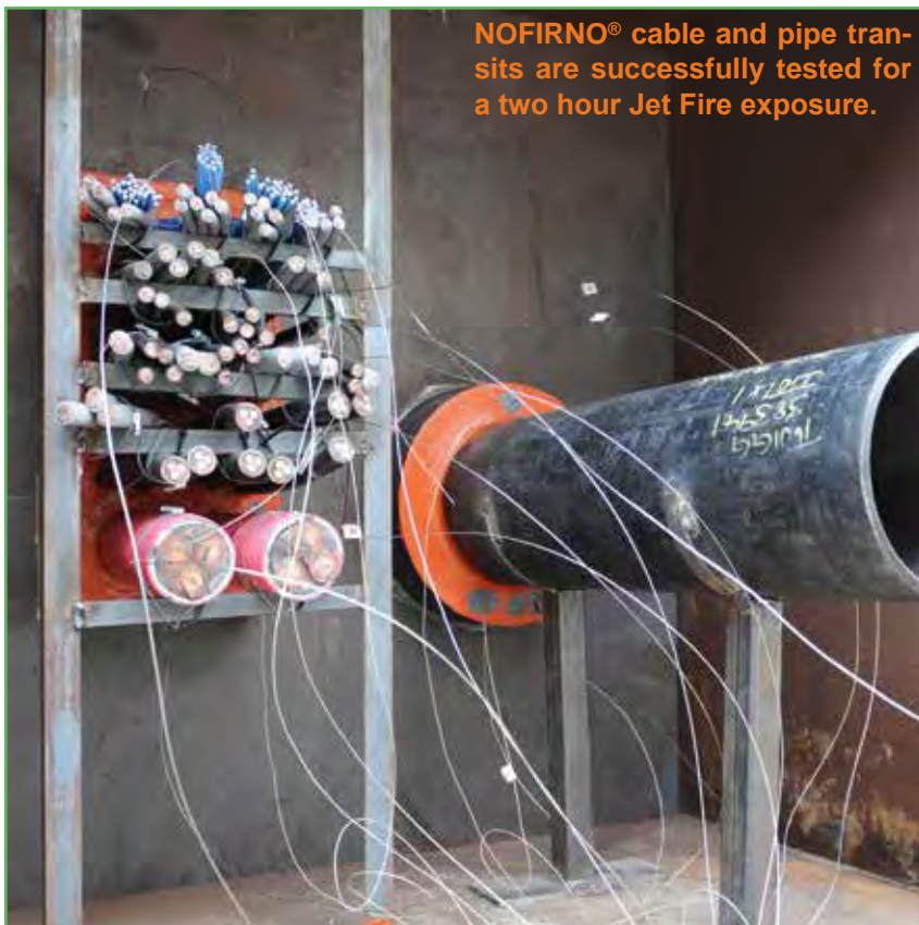
In some areas, in the flame temperatures of 1200 °C are reached. Heat flux vs. black body temperature: 250 kW/m 2 equals 1175 °C.
